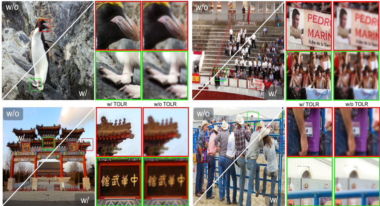
Figure 5. Deblurring results comparison of deep optics with and without tolerance-aware optimization under tolerances perturbations. The deep optics with tolerances optimization maintain better deblurring performances than its counterpart.
