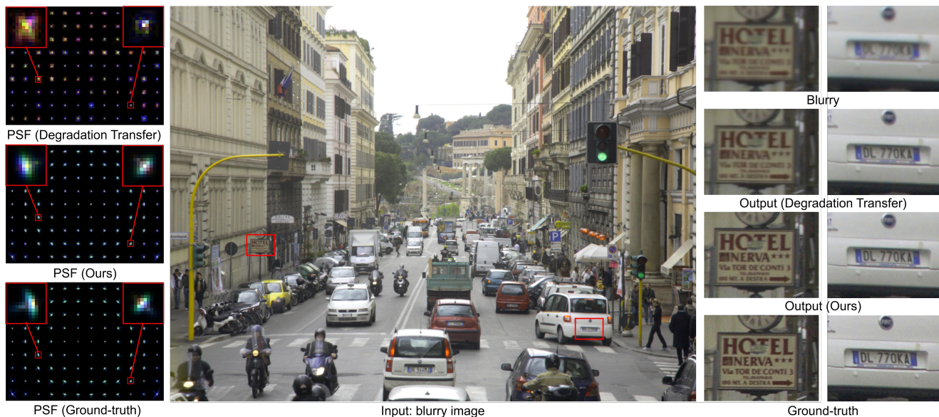
Figure 1. We introduce a point spread function (PSF) estimation framework and demonstrate its effectiveness in deblurring. From left to right: PSF estimated via Degradation Transfer [6] (state-of-the-art), PSF estimated by our method, and the ground-truth PSF of lens #63762 from Edmund; a blurry input image synthesized using an image from the FiveK dataset [5] and the ground-truth PSF; the patches from the blurry input image; the patches deblurred by pre-trained Restormers [46] using training data generated from PSFs obtained through our method and Degradation Transfer [6], respectively; and the corresponding ground truth patches. Our approach outperforms existing state-of-the-art methods in both PSF estimation accuracy and deblurring quality.
