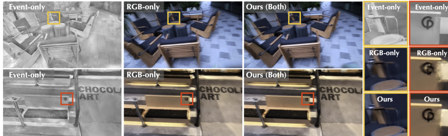
Fig. 6: Qualitative ablation on input modalities. Event-only reconstruction captures fine-grained structural details but lacks color information. RGB-only reconstruction preserves color fidelity but suffers from severe blur artifacts. Ours (Both) combines both modalities, achieving sharp details with faithful color reproduction. Zoom-in patches (right) highlight the complementary strengths of each modality.
